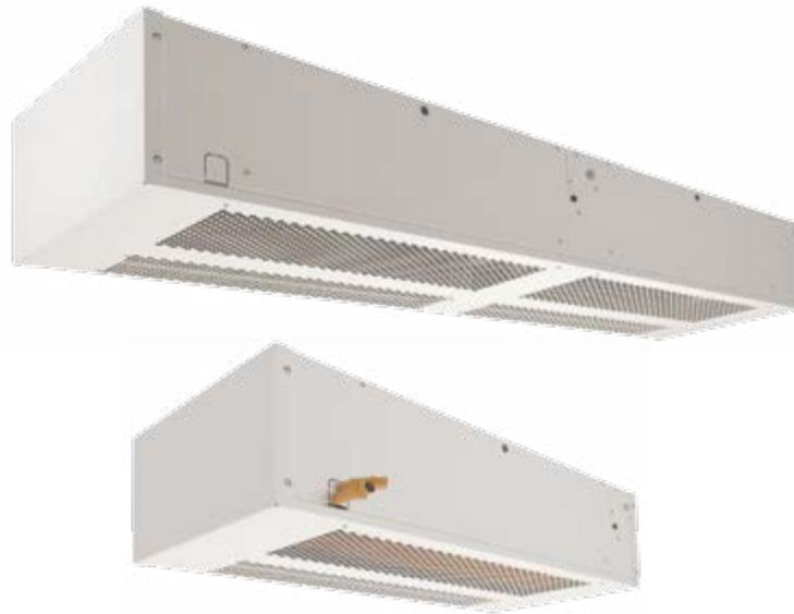
Series 301 - Designed specifically for installations into standard drop ceilings of up to 11' (3.5m) in height, but can be utilized wherever a flush mounted air curtain will be required for commercial, retail or institutional applications. Can be secured directly to structure from above or suspended on chains or threaded rods.
