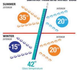
HPS-G HeatShield uses the solar bands of light and converts them to heat in the window.
